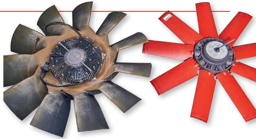
173.9kW/233.2hp, but again inside measurement tolerance. Things were much the same with specific fuel consumption: before and after values were 248/247g/kWh at rated speed, and 234/233g/kWh at max power. So there was no significant improvement at two key points on the full load curve. However, both power and fuel consumption did benefit from the Cleanfix fan below 1,400rpm, which in some work would be useful.
