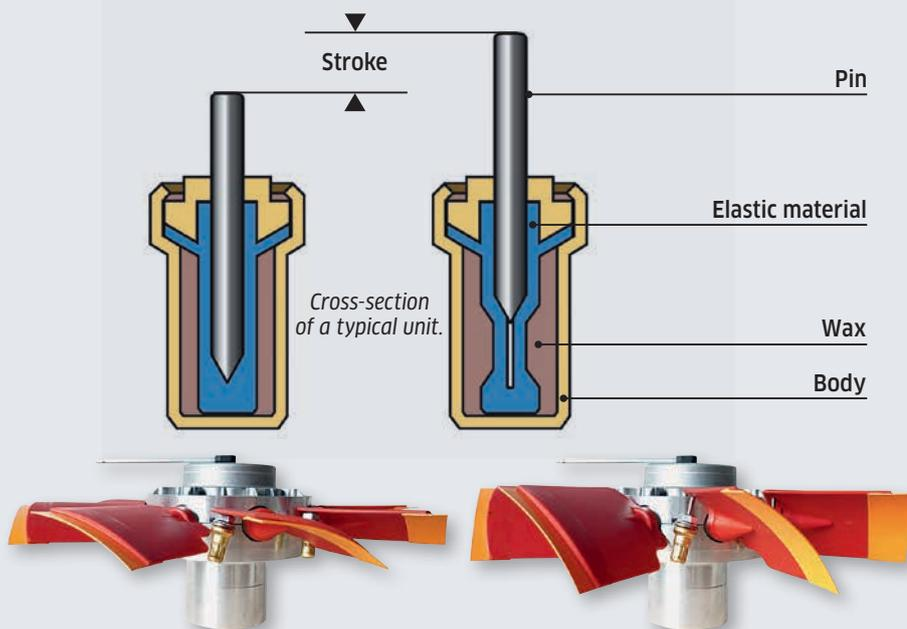
Below the actuator's threshold temperature, blade angle is at minimum and the actuator pin retracted.
