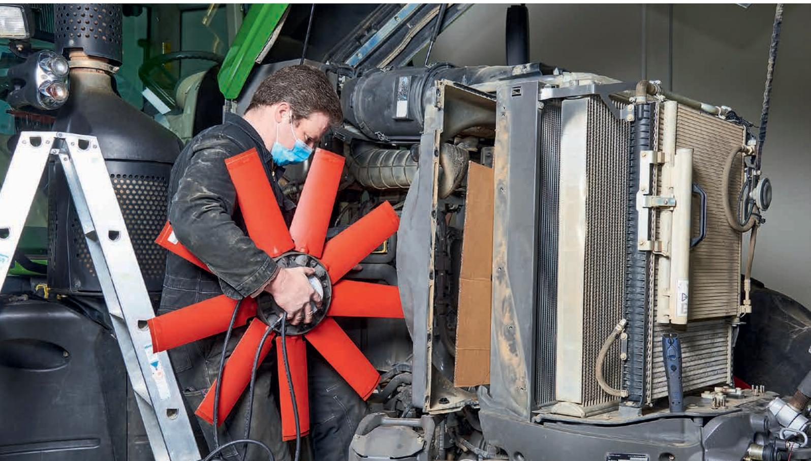
*He's a big fan. Retrofitting a Cleanfix unit isn't necessarily difficult but can take a while. To see the effect we asked the DLG to measure pto power and specific fuel consumption on New Holland and Fendt tractors, before and after fitting. Photos: Uhlig.*
