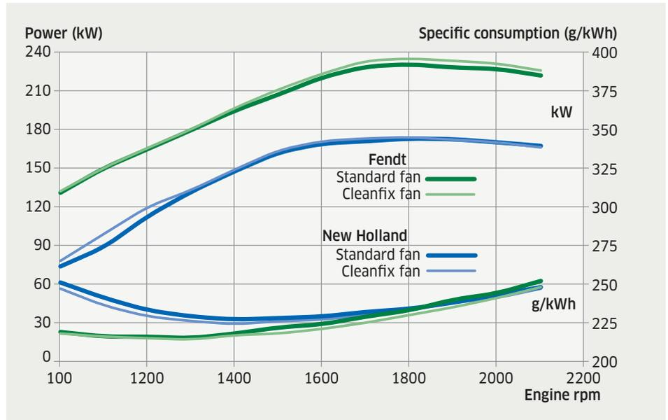
With the New Holland T7.270 the Cleanfix fan has little effect beyond 1,300rpm. Fendt's 936 Vario benefitted more, showing higher power and lower fuel use at both rated and max power rpm. Graph: Tovornik.
