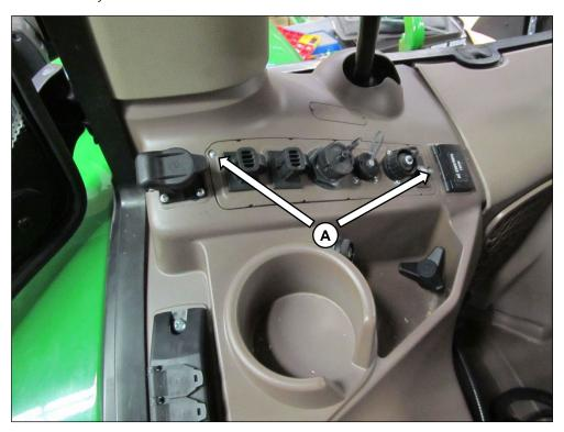
Lift out and remove the cover plate for the switch from the connector holder.
