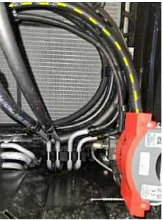
► Connect the pressure hose to connector A of the Cleanfix® valve unit.
