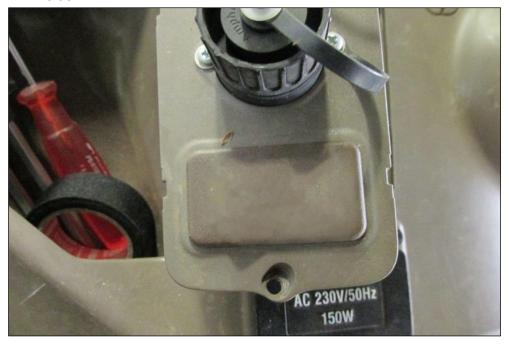
Remove the screws on the socket.
