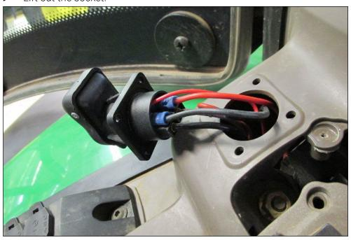
▶ Remove the cover below the connector holder.
