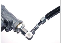
Run the pressure hose with corrugated tube as shown.
