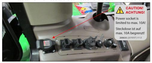
► Attach the Cleanfix label above the switch.
