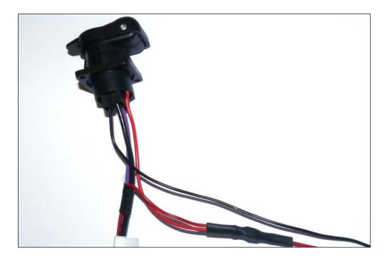
Reinstall the socket and connector holder.
