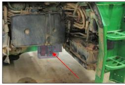
The attachment points provided for the compressed air system can be used for attachment. ► Use suitable screws to install the bracket for the Cleanfix® control unit.
