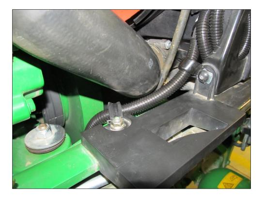
► Use the supplied rotatable cable clips to attach the corrugated tube with pressure hose to adjacent cables or pipes.
