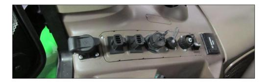
Attach the Cleanfix label above the switch.
