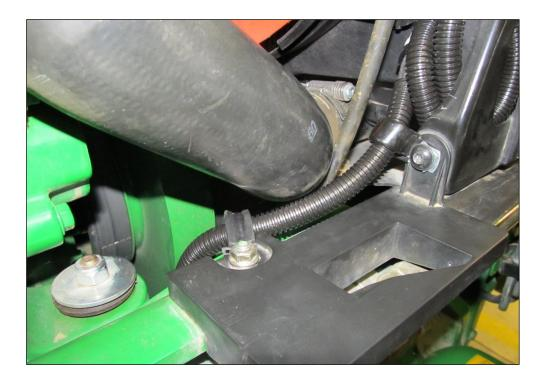
▶ Use the supplied rotatable cable clips to attach the corrugated tube with pressure hose to adjacent cables or pipes.
