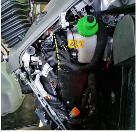
► Connect Superseal connector to freely available 4-pin Superseal connector.
