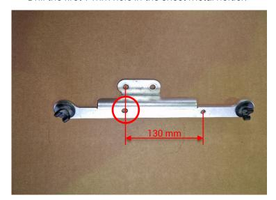
► Drill the second 7 mm hole in the sheet metal holder at a distance of 130 mm.
