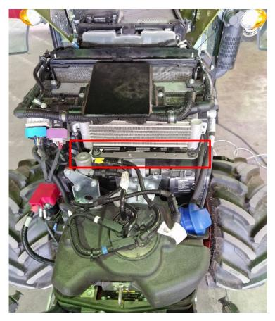
▶ Drill the first 7 mm hole in the sheet metal holder.
